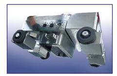
This view of the underside shows the enclosed port (center) for the downward-looking laser scanner and video camera, as well as the four independently powered and steerable drive wheel pods.
