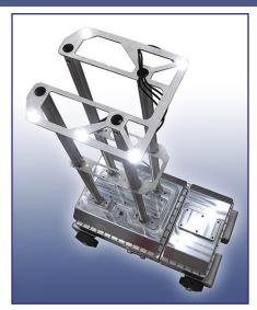
**Mast-top mounted LED lights** enable the precision navigation global positioning camera, mounted on a boom inside the tank hatch, to track the robot. The mast height keeps the LEDs above any sediment and turbidity.
